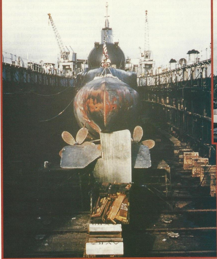
Drydocked at Pearl Harbor the TUNNY reveals the size of her five-bladed high speed propellers, stern diving planes and rudder.
